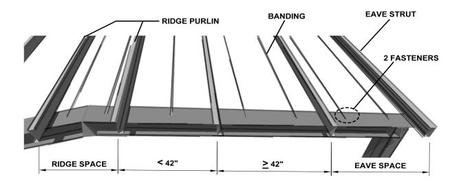
Bi-Directional Banding Providing OSHA-Compliant Leading-Edge Fall Protection
