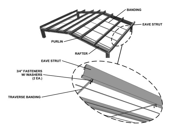
4. Pull each band hand-tight towards the ridge purlins while weaving above every  $7^{th}$  or  $8^{th}$  longitudinal band and above the bands in the ridge space. Fasten to the ridge purlins and far eave strut using one (1) of the  $\frac{3}{4}$ " TEK 3 fasteners with washers provided. **Do not fasten into purlins at this point.**
