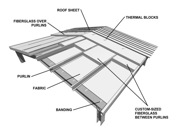
Bi-Directional Banding Providing OSHA-Compliant Leading-Edge Fall Protection
