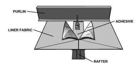
Bi-Directional Banding Providing OSHA-Compliant Leading-Edge Fall Protection
