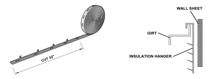
5. Two (2) hangers should be used to hold any insulation blanket up to 72" wide by placing them 18" from each side of the insulation blanket (or 36" apart). Repeat this step for each wall area to be insulated. Hangers not supplied for girt spaces 24" or less.
