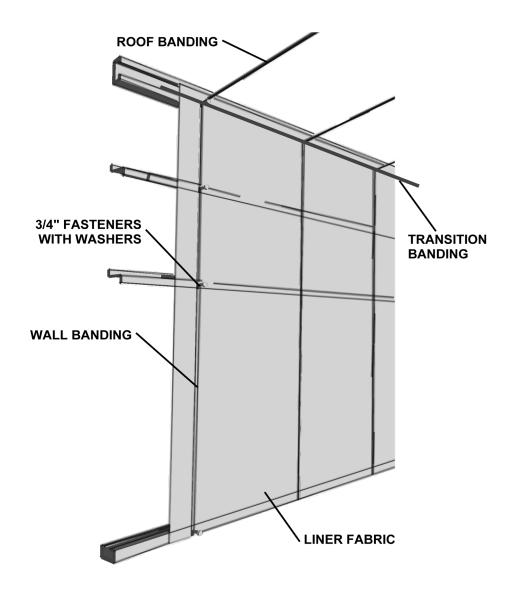
a. NOTE – Every effort should be made to connect the ProLiner<sup>™</sup> roof and wall fabric for a tight building envelope seal. Additionally, fabric edges should be properly sealed to adjacent surfaces to maintain vapor and air barrier integrity.
